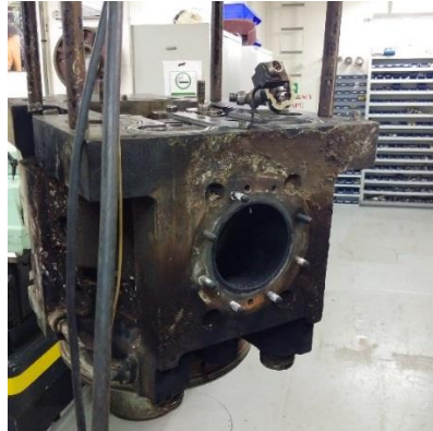
Damaged cylinder cover, exhaust gas side
