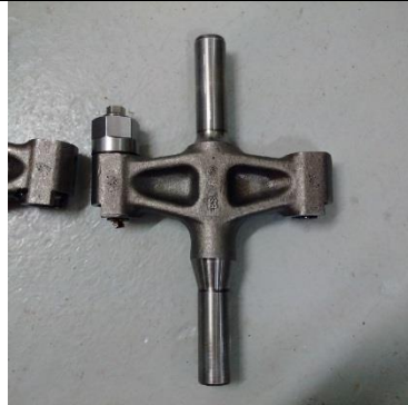
Bended spring pusher for inlet valves
