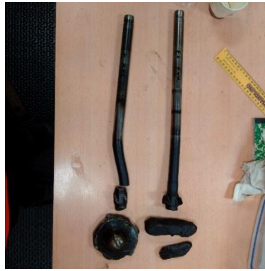
Damaged exhaust gas valves
