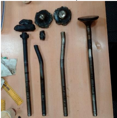
All 4 damaged valves
