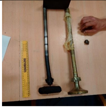
Damage exhaust fore and new valve
