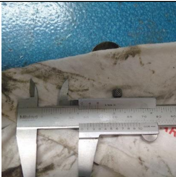
Measured 27 mm cam height
