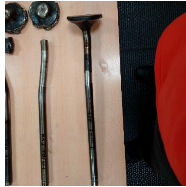
Damaged air inlet valves
