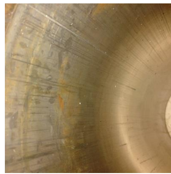
More scratches on cylinder liner
