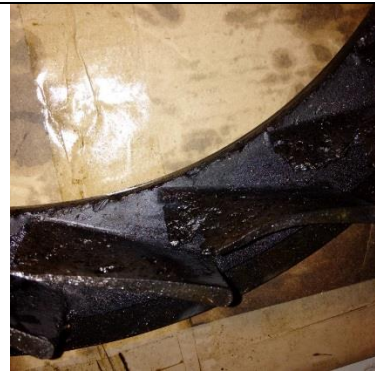
Damaged turbine nozzle
