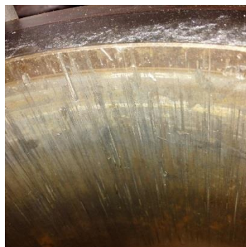
Scratches on cylinder liner
