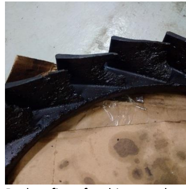
Broken fins of turbine nozzle
