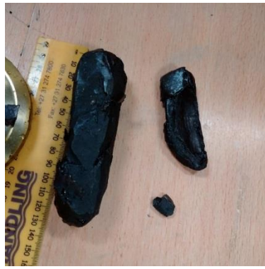
2 main parts of forged valve's crown
