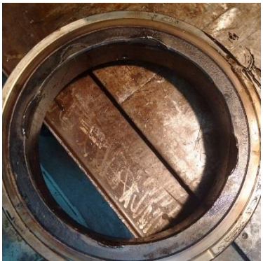
Damaged topland ring, top view
