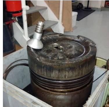
Damaged piston with broken piece of connecting rod
