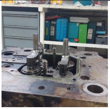
Damaged cylinder cover with spring pushers
