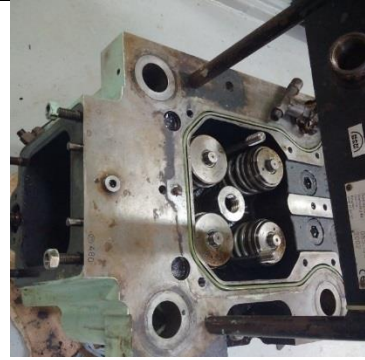
Damaged cylinder cover side view
