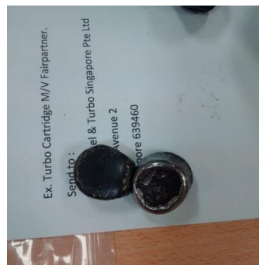
Broken parts from piston middle area
