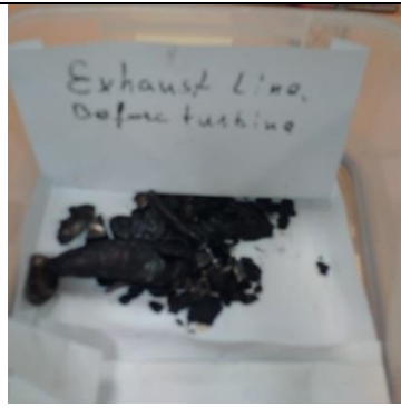
Detached pieces found in exhaust manifold
