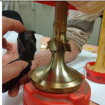
Detached fins piece from exhaust rear valve
