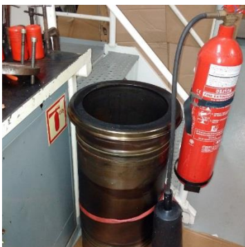
Damaged cylinder liner
