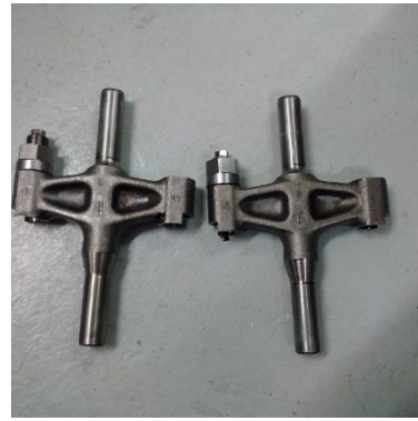
Valves opening pushers, slightly deformed
