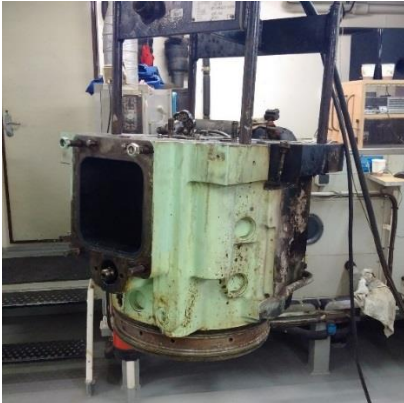
Damaged cylinder cover, charging air side
