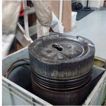
Damaged piston, side view
