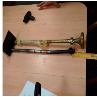
Comparison of damage exhaust forward valve with new one
