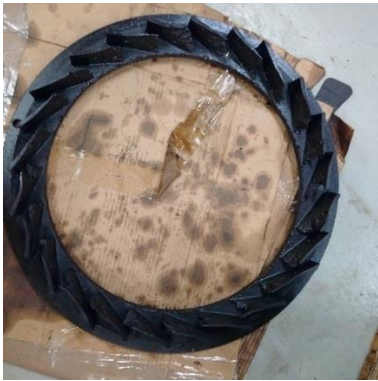
Damaged turbine nozzle
