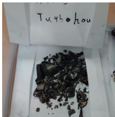
Parts found inside turbine housing
