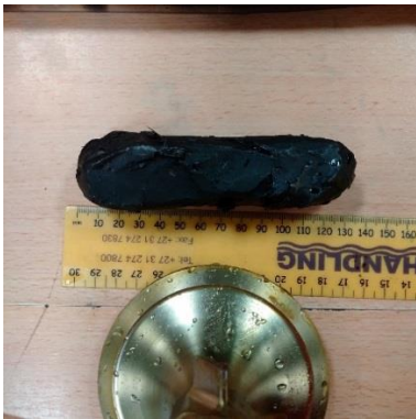
Bigger part of exhaust forward broken crown
