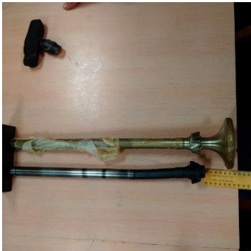
Damaged exhaust forward valve and new one
