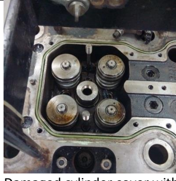
Damaged cylinder cover with stems in place
