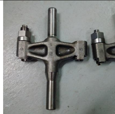
Bended spring pusher for exhaust valves
