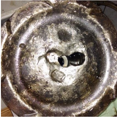
Damaged piston, top view
