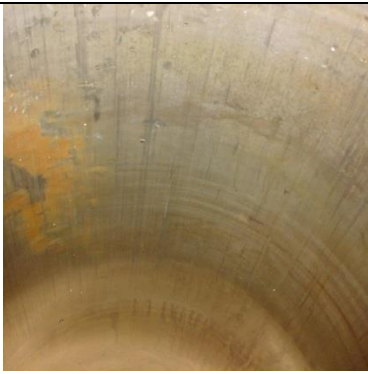
Scratches on cylinder liner
