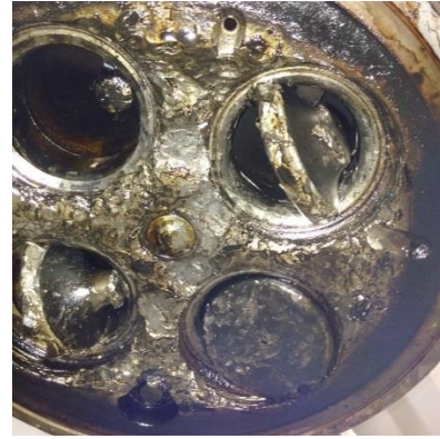
Valve crowns broken and rotated
