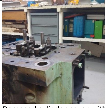
Damaged cylinder cover with pushers, side view
