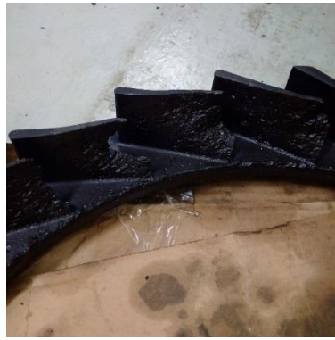
Damaged fins of the nozzle
